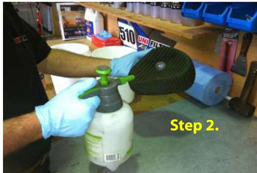
**Step 2.** After putting on the latex gloves, pour the “Filter Cleaner” into the pressure spray bottle and spray the dirty filter both inside and out. Massage the cleaner through the filter.
