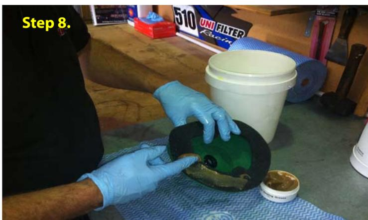
**Step 9.** The filter is now cleaned & re-oiled ready for use.
